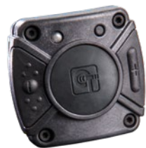
CT-WirelessPTT MIL with PPT button curved outward
